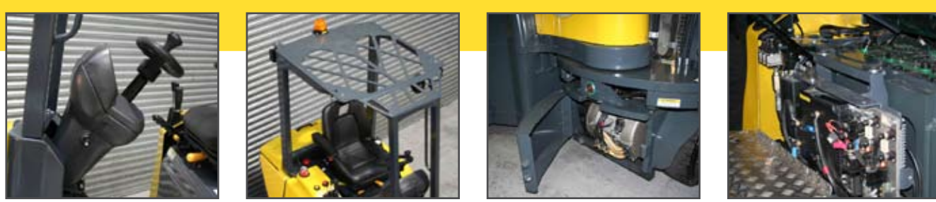
Adjustable Steering Column 4 Post Overhead Guard 19.5kW AC Motor Ease of Access
