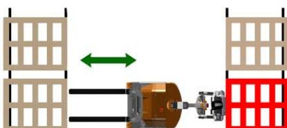
Standing to the side of the stacker eliminates the risk of being trapped or crushed while allowing the Combi-CS to operate in very narrow aisles.
